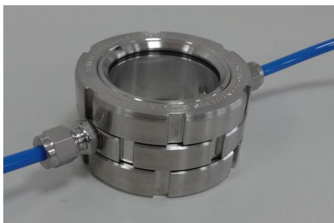
**Figure 1.** Custom-built UV irradiation chamber with CaF<sub>2</sub> windows, suitable for inert atmospheres
