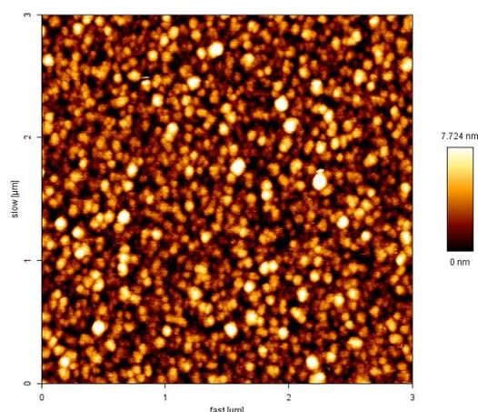
**Figure 2.** AFM image of fluoropolymer thin film following exposure to 254 nm UV radiation for 21 h
