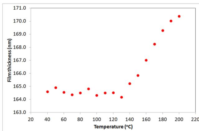
**Figure 2.** Thickness of a PMMA film as a function of temperature, showing  $T_g$  around 130 °C
