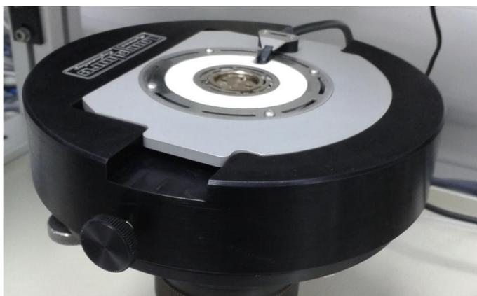
**Figure 1.** UVISEL ellipsometer modified with a custom adaptor, securely housing a high temperature heating stage
